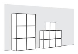
With now! easy it is possible, to stack assembly units. In this case a wall bracket must be ordered for each stacked unit.
